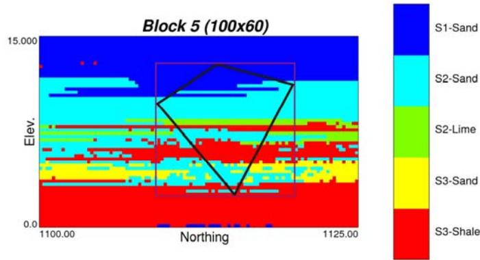
**Figure 6.** An irregular grid is imposed on a heterogeneous medium (see Paper 206 for construction of this facies model).
