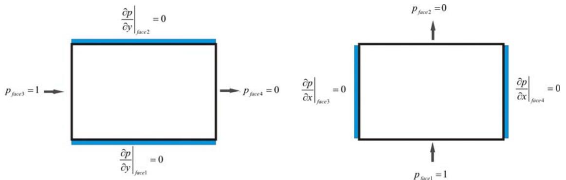
**Figure 3.** Boundary conditions applied on coarse grid when flow is in  $x$  direction (left) and  $y$  direction (right). Thick blue lines indicate no flow boundaries on those edges.
