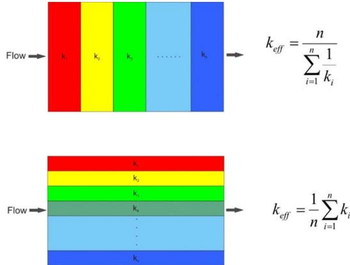
**Figure 1.** Upscaled effective permeability for simple cases of series (top) and parallel (bottom) layers. Redrawn from Kelkar and Perez (2002).
