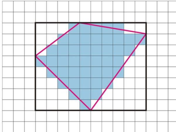
**Figure 4.** A diamond shape coarse grid and the underlying fine scale model. Shaded fine scale blocks lie inside the coarse irregular grid and are considered for the calculation of effective permeability. The rectangular region (dark black line) is the smallest rectangle that will encompass the irregular grid.
