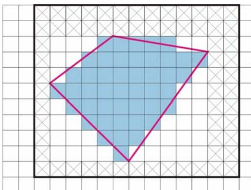
**Figure 5.** An unstructured grid with the buffer zone around it. Size of buffer zone is controlled by four integer values which indicates how many cells should the smallest rectangle be expanded on each side (2 from top, 1 from left, 2 from right and 1 from bottom).
